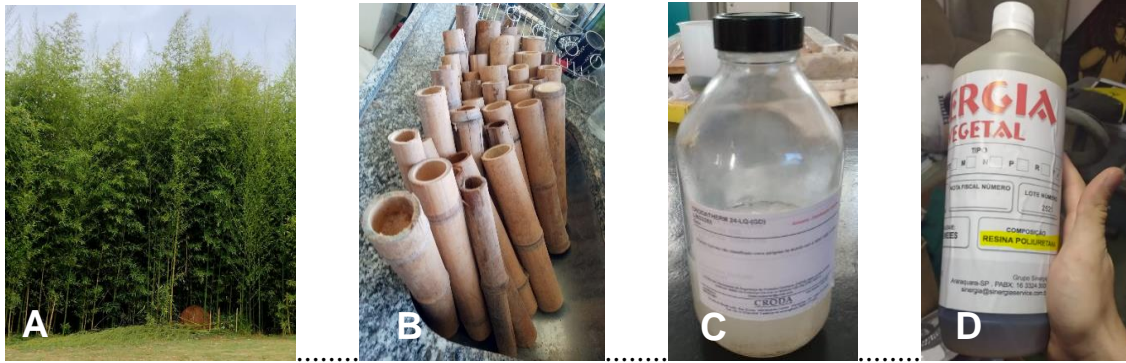
Fig. 2. Materials used in the research: (A) Clump of Phyllostachys aurea where the research material was harvested, (B) Pieces of bamboo culms used, (C) Commercial CrodaTherm 24 PCM, and (D) Resin used for sealing PU VEGETAL – TYPE "V" commercial.
