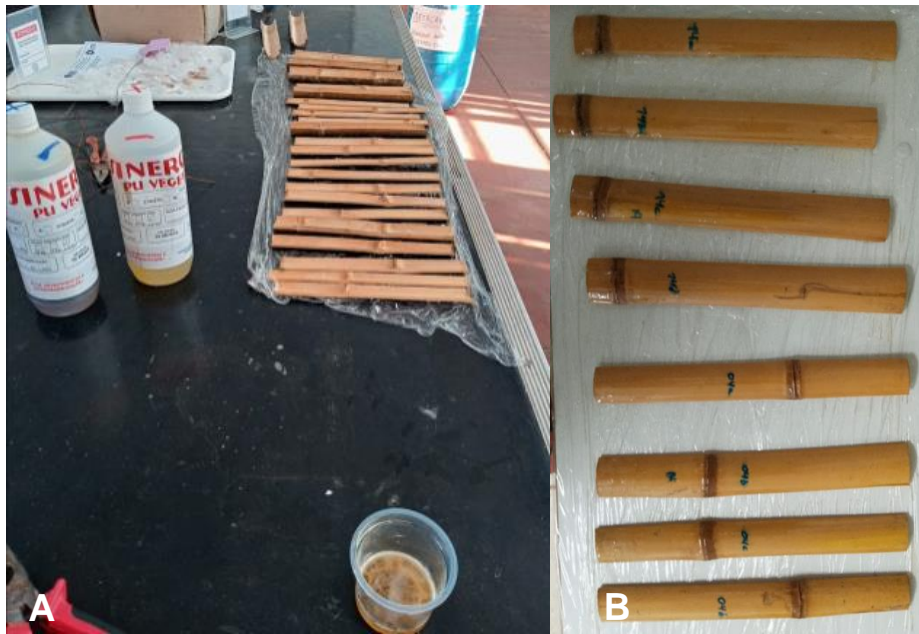
Fig. 5. Two-component PU mixture for application (A) and the systematization for application (B).
