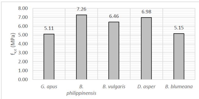
**Fig. 10.** Characteristic shear strength parallel to fiber ( $f_{v,c}$ ) (Bautista et al. 2021).
