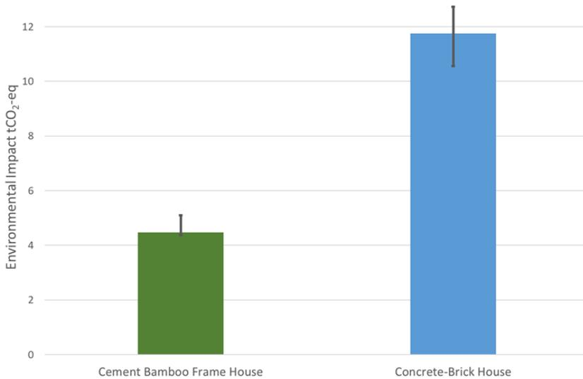
**Fig. 13.** Comparative Life Cycle Assessment between cement-bamboo frame house and conventional concrete-brick house (Escamilla et al. 2022).
