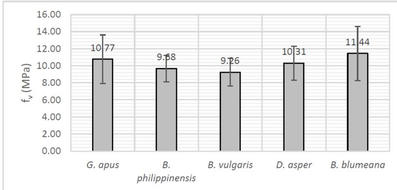
**Fig. 9.** Average shear strength parallel to fiber ( $f_v$ ) (Bautista et al. 2021).
