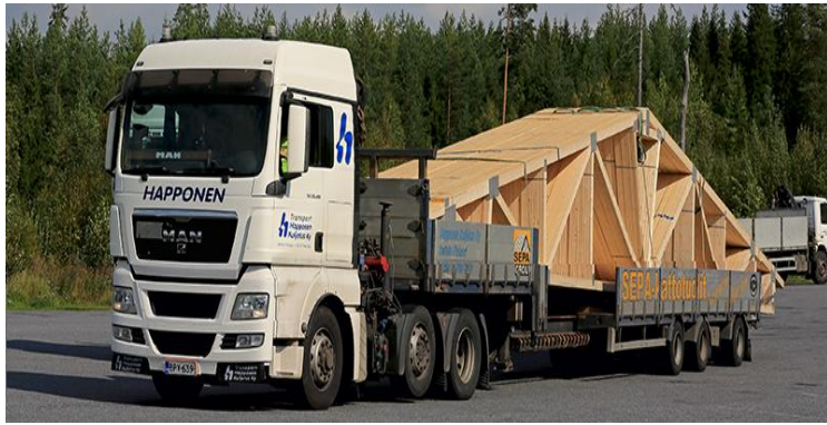
Level 1 - Truss components
