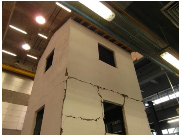
Plate 10: Unidirectional shake table test on two storey house at the University of the Andes, Colombia (Arup & Imperial College, 2013[21])
