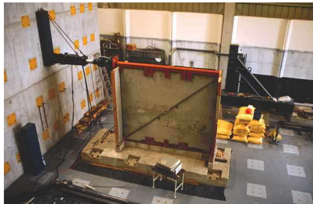
Plate 8: Cyclic load test on structural Bahareque , in Costa Rica (Gonzalez and Gutierrez, 2003[18])
