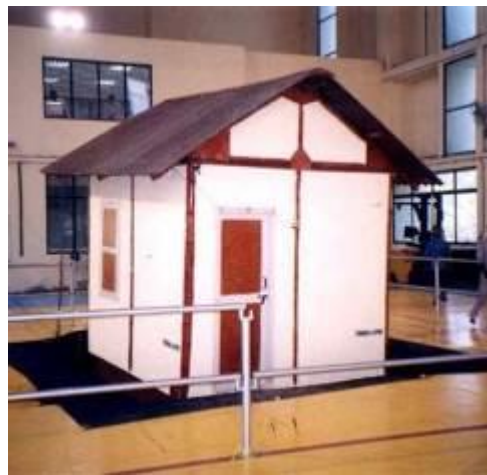
Plate 14: Bamboo house under shake table testing at CPRI, Bangalore [1]
