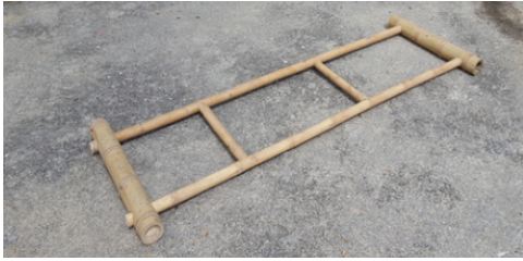
Base chassis construction (Figure 34)
