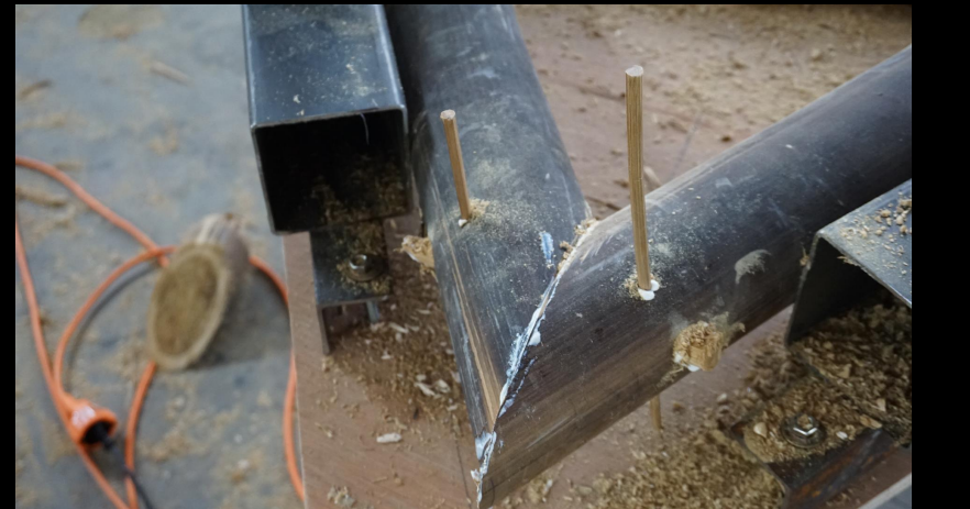
CORNER CONSTRUCTION: Filled ends, parts built in jigs with modern tools, large dowel with smaller cross pinning of dowel
