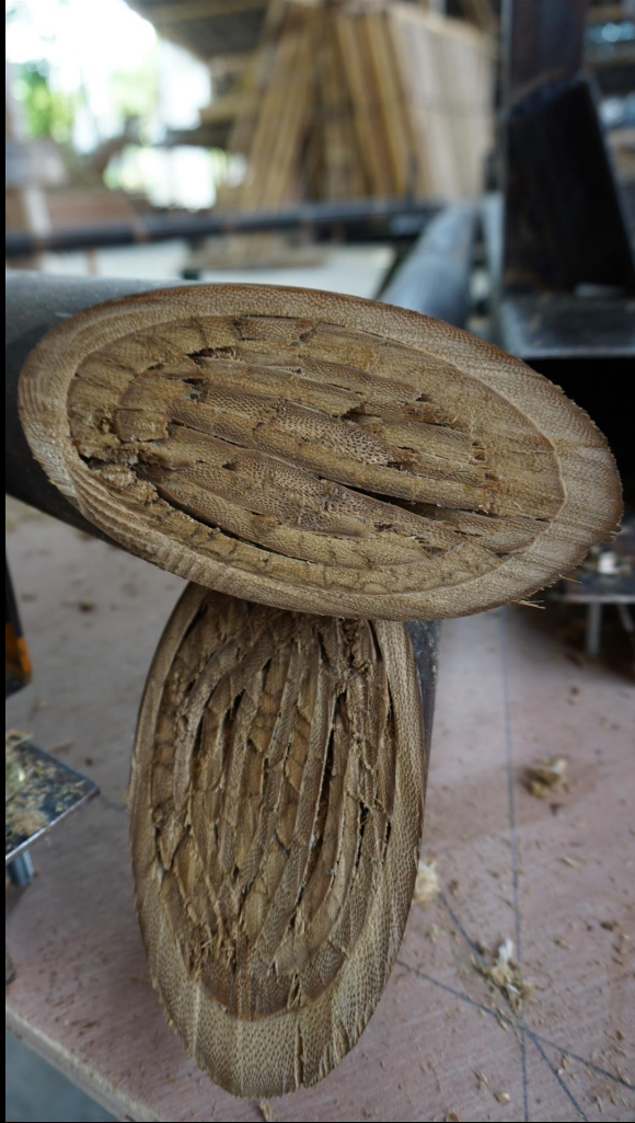
CORNER CONSTRUCTION: Filled ends, parts built in jigs with modern tools, large dowel with smaller cross pinning of dowel
