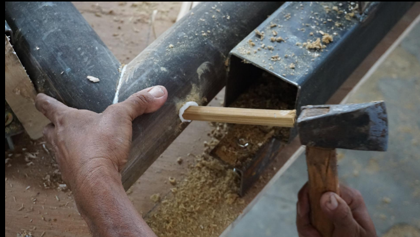
CORNER CONSTRUCTION: Filled ends, parts built in jigs with modern tools, large dowel with smaller cross pinning of dowel
